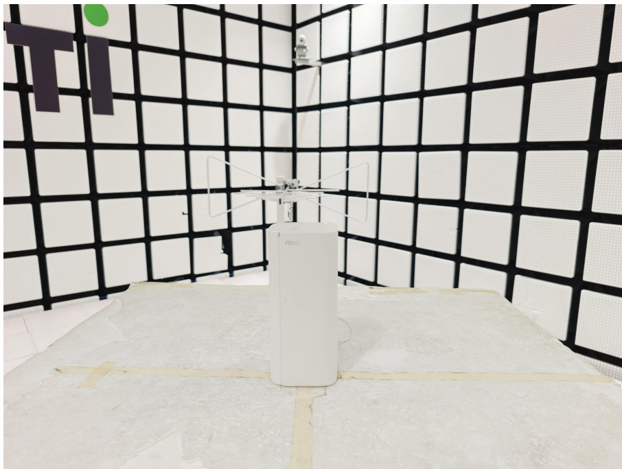
Radiated spurious emission Test Setup-1(Below 1GHz)
